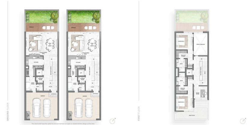
Adjoining townhouse plans: the same layout mirrored. The end unit gains a side garden and windows on a third façade.
